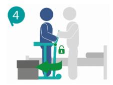
The assistant unlocks and rotates the turntable smoothly left or right to engage the brake rod into one of the five locking positions.
